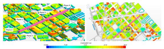
Figure 3. Planes used for street ventilation assessment (l.h.) and street orientation (r.h.).
