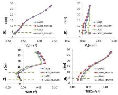
Figure 3. Vertical profiles of average flow properties over the study street. a) wind speed normal to street  $(V_n)$ ; b) wind speed parallel to street  $(V_p)$ ; c) vertical wind speed (W); and d) turbulent kinetic energy (TKE). Dashed lines indicate new trees location.
